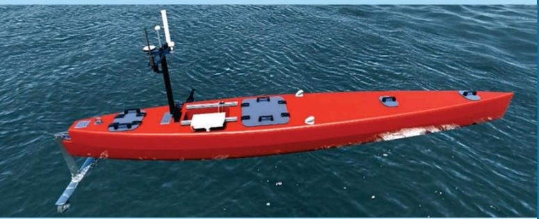
As part of 'VISION 2030', GRSE is witnessing a paradigm shift in its R&D effort to develop Unmanned Surface Vessels with the application of Artificial Intelligence and Machine Learning. As a first step, GRSE developed a 5m Autonomous Surface Vessel named as Swadheen a ground up based design for bathymetric surveying, mine-hunting and explosive ordnance disposal.
