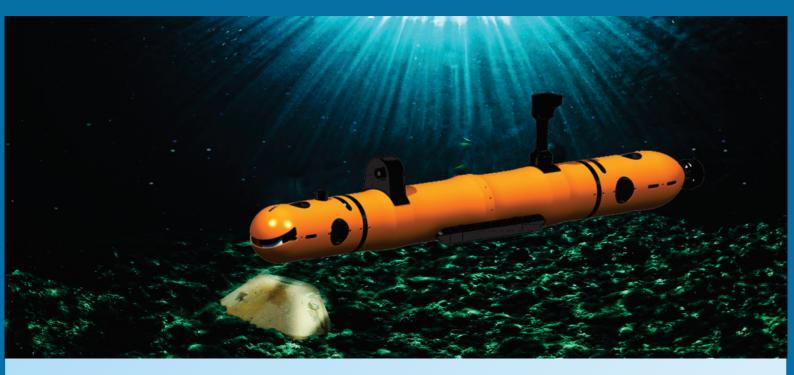
Autonomous Underwater Vehicle (AUV). GRSE in collaboration with an industry partner M/s AEPL has developed a Man Portable AUV (which is being launched today). The AUV has been designed as a completely autonomous vehicle and is designed to take on a variety of payloads depending on the required role including mine detection, ASW training, underwater inspection, search & rescue missions and scientific exploration.
